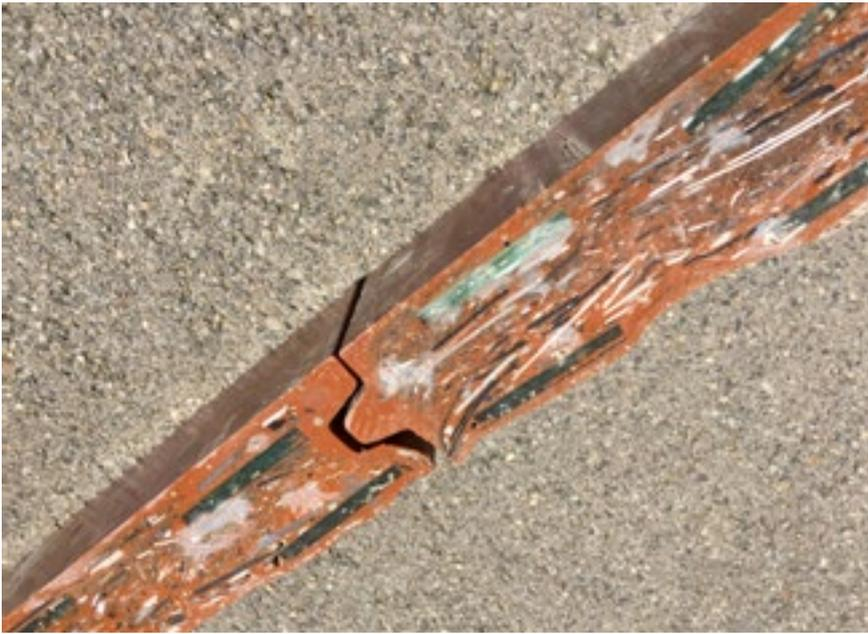
At the Beatrix lock-gate in Almere, The Netherlands the 80 profiles were used to install a camp sheeting. The placement process, vibrating the profiles into the soil with a hammer block was experienced by the crane operator to be as easy as with the traditional profiles made of tropical hard wood.
